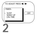
Press the PLAY/▲ button or the STOP/▼ button to select SLEEP. Then press the REW(ind)/◀ button or the F.FWD/▶ button to select 30 MIN(utes), 60 MIN(utes), 90 MIN(utes), or 120 MIN(utes). (You can not set the sleep timer during a recording.)
